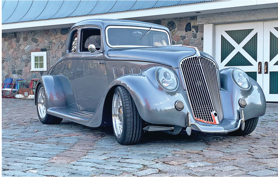
The Veit Foundation’s 1933 Willys Coupe Model 77 was built by Dave and Lisa Simard of East Coast Customs. The car is powered by a 3.8-liter Grand National Turbocharged engine, has highly customized wider fenders and a full custom chassis.
